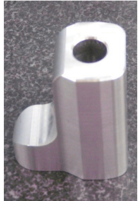
Compensator for a 9mm pistol, machined from 7075 aluminum using a VoluMill™ toolpath.
