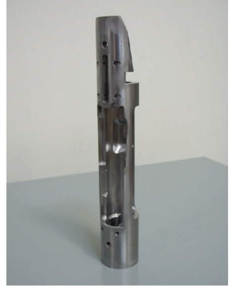
VoluMill™ toolpaths were used to machine this receiver for McMillan’s famous .50-caliber BMG 50 rifle.
