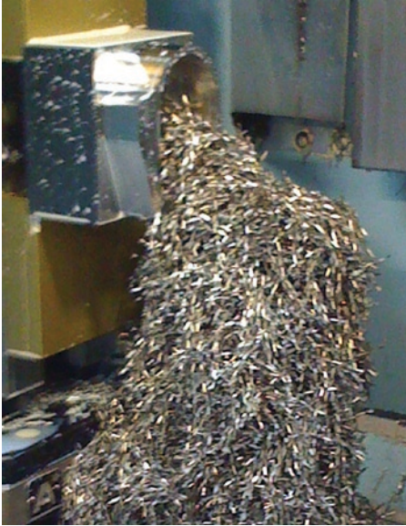
A VoluMill™ toolpath in the process of reducing a 28-pound block of 17-4 stainless steel into a 2.8-pound weapon-mount component.
