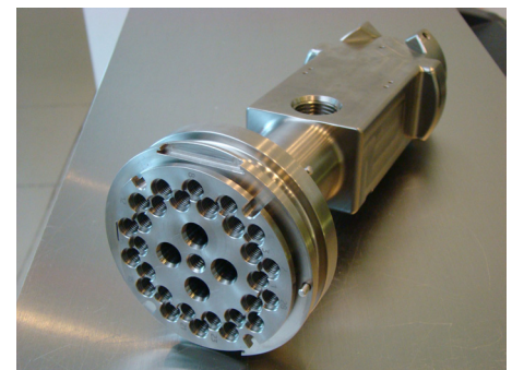
This Titanium energy industry component took 18 minutes to rough using a traditional toolpath and only 11 minutes using a VoluMill™ toolpath.
